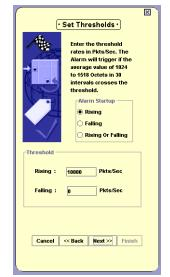
Figure 6-6. Alarm Wizard - Set Thresholds
